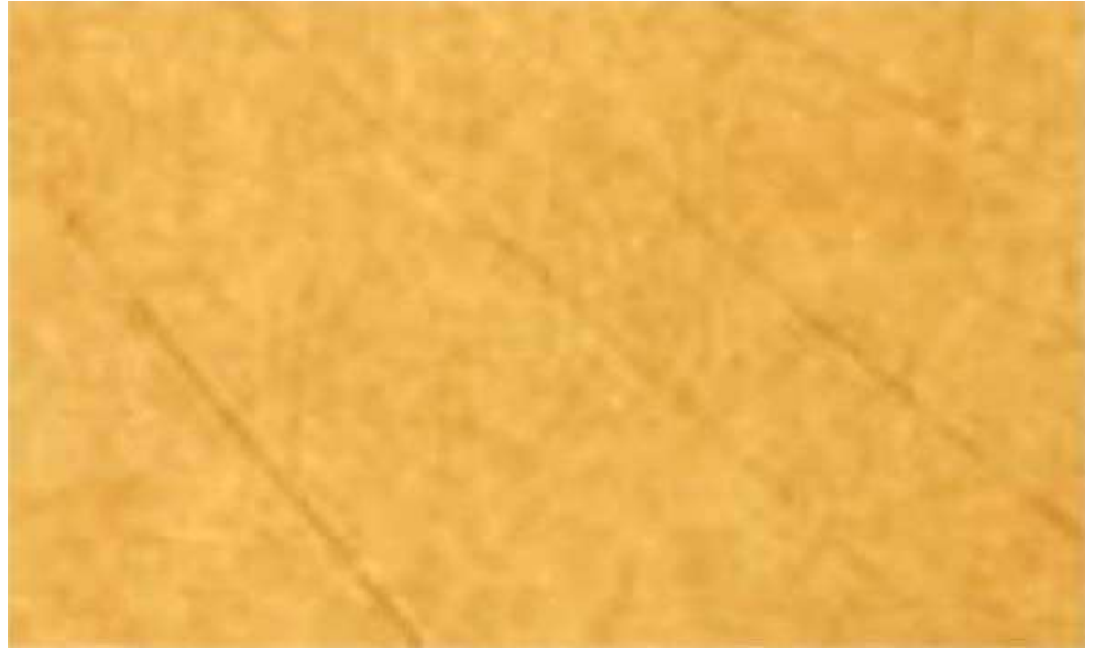
Figure 6.6.18 Scratches on FRP Surface
